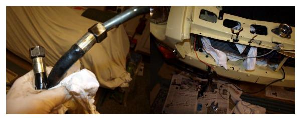
Yes a messy job, <u>but</u> the unintended consequence of the task - which I am really fortunate to have undertaken - was that the rubber oil cooler pipes I removed had almost <u>PERISHED</u>.... and the rubber was badly cracked where it sits underneath the body slam plate and where
