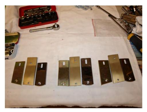
Look at the photograph, our three originals are in the middle of each group of three. Fitting the new replacements (tried both types) onto the grille and back towards the slam panel to get the grille back in place on the nearside wing curvature meant the bonnet wouldn't close against the central MG Grille Motif. Perhaps the MGC has a different spacing between its MGB common Radiator Grille and the MGC slam panel so the parts are being incorrectly sold as "fitting both an MGB and MGC's?
